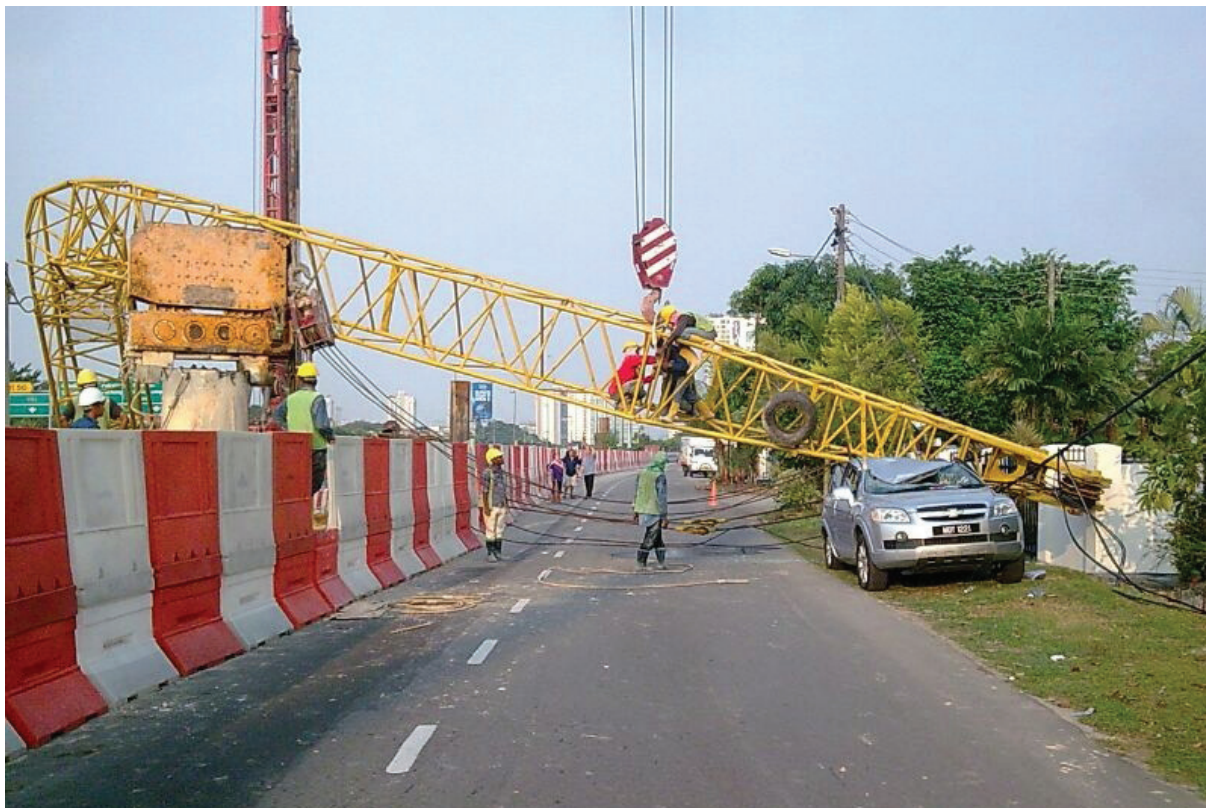
Photo 2.0: The crawler's lattice boom structure failed and landed on the car.
