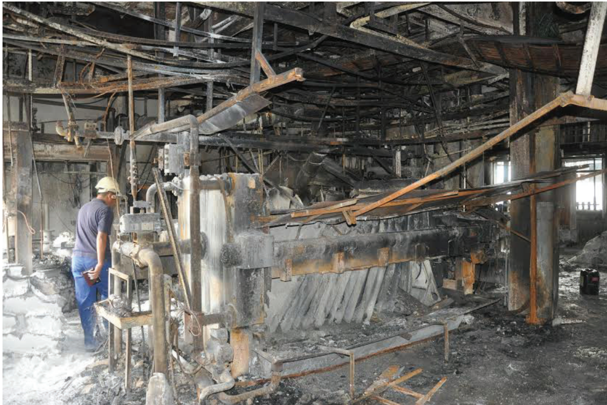
Photo 3.0: Scene after the explosion and fire in the MgSt and ZnSt processing plant.
