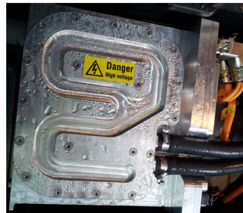
Condensation at outer surface of on-board charger
