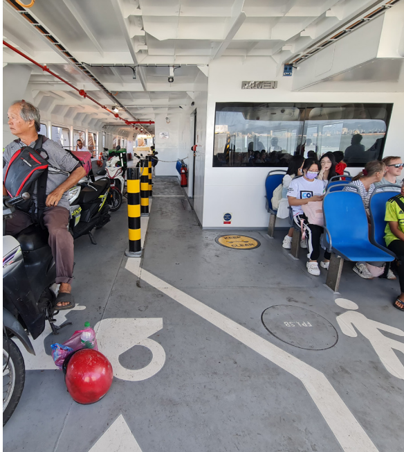
Photo 8: Inside the new ferry, passengers and vehicles are separated by the cabin wall.
