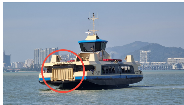
Photo 4: Docking platforms fitted to the new ferry. These functioned as gates when raised upon complete embarkment.
