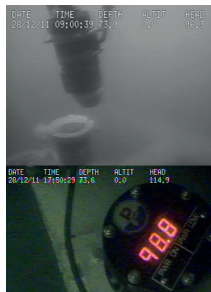
Figure 2: Subsea valve closing/opening using a subsea torque tool.
