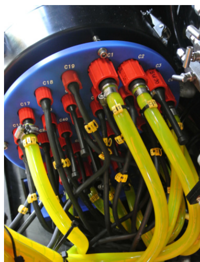
Figure 9: Work class ROV with MCP installed. Right photo shows the end cap of the MCP with all the subsea cables (whips) connected to various ROV functions.
