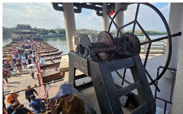
An exhibit on site shows the winch used in earlier days to manoeuvre sets of boat pontoon during the opening and closing stages.
