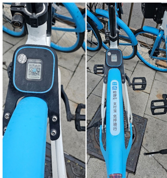
Photo 2: The QR code is a convenient way for users who log in to unlock the bicycle and log out upon arrival. The system will then compute the charges.
