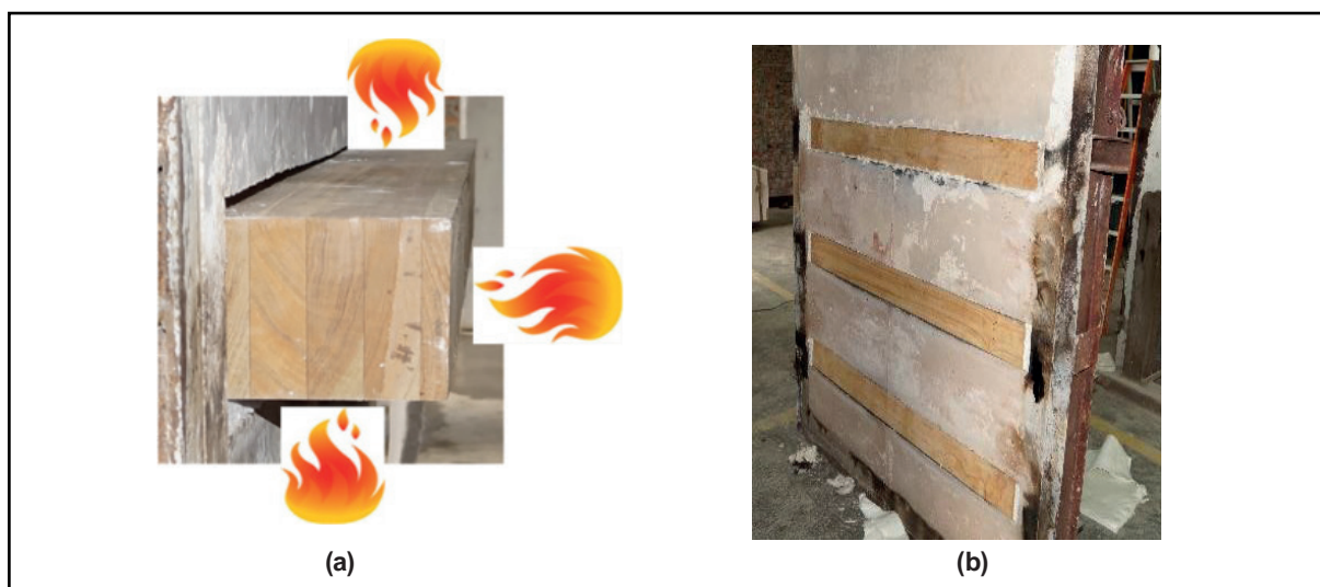
Figure 7: Mounting specimens on test frame flush with cement; (a) 2-D samples and (b) 1-D samples
