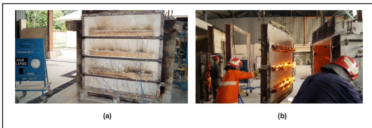
Figure 8: Actual fire test set-up: (a) 2-D specimens with attached thermocouples and (b) specimens after fire test
