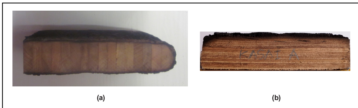
Figure 9: Examples of the conditions of the samples after fire exposure: (a) glulam and (b) LVL
