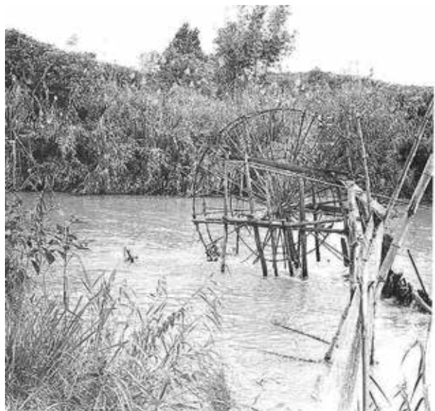
Undated photo showing a wooden waterwheel propelled by the current lifting river water into the adjacent bamboo channel to be transported to the paddy field nearby.
