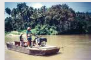
Boat being propelled by river current to the opposite river bank
