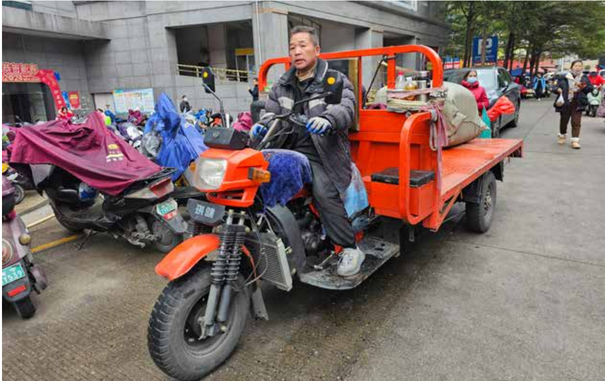
Photo 7: The more powerful petrol engine type. This model is driven by a 125hp engine and is used to carry heavier loads for short-haul within the mid-tier city of Nanning's old town goods dispatching centre in Guangxi province. Notice the double shock absorbers at the front wheel to cope with the heavy load it carries. (Photo courtesy of Huang Zhaoliang of CMQIP)
