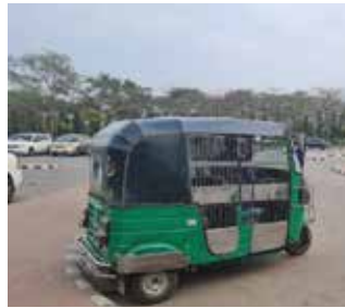
Photo13: The above passenger tricycles used in Bangladesh are either powered by LPG or battery. (Photo courtesy of Ar Dr Goh Ai Tee).
