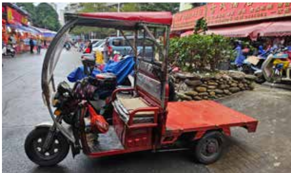
Photo 4: This flat-bed type, powered by a battery kept below the seat of the driver with a rooftop that offers shelter against rain, is useful in areas with frequent rainfall.
