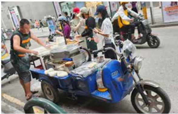
Photo 3: The simplest type of tricycle pickup is a small open-cabin single-seat vehicle with motorcycle handlebars and a small pickup box at the back. The photos show a hawker selling breakfast on a Guangzhou street. It moves about the commercial area to catch the morning office staff coming out of subway stations en route to their offices. This particular pickup is driven by a petrol motorbike engine although more people are converting them to a battery-driven type.
