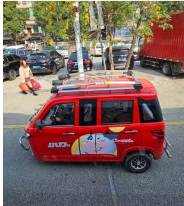
Photo 11: Modified tricycle with cabin for two passengers or goods that need to be shielded from rain and sun.
