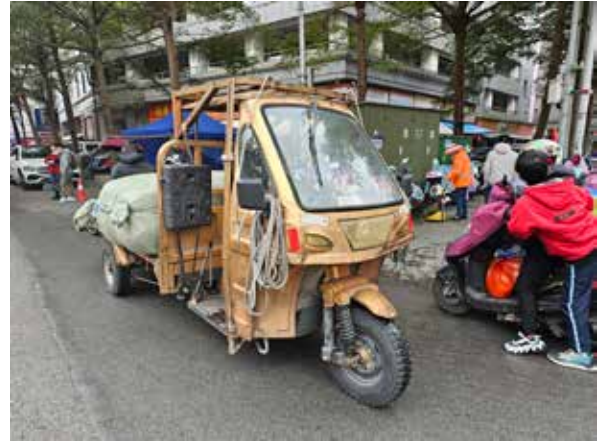
Photo 5: This cabin-enclosed type offers complete shelter from rain and with a bigger loading capacity. Notice the brake handles and the wheel lock system in front of the carriage vertical bar just behind the driver seat. The loading capacity depends on the motor engine capacity. The wheel size is also bigger than a normal motorbike to cater for heavier loads.
