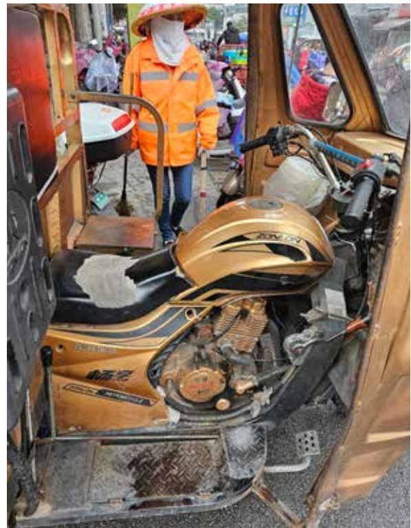
Photo 6: Interior view of the bike handle of another similar type but without a door. Notice the foot braking system, petrol tank and simple outfit that makes maintenance easier and more cost-effective.
