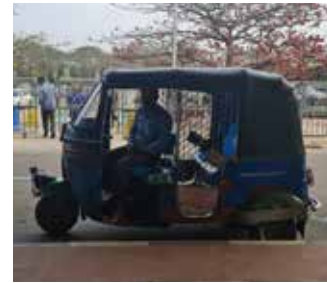
Photo13: The above passenger tricycles used in Bangladesh are either powered by LPG or battery. (Photo courtesy of Ar Dr Goh Ai Tee).
