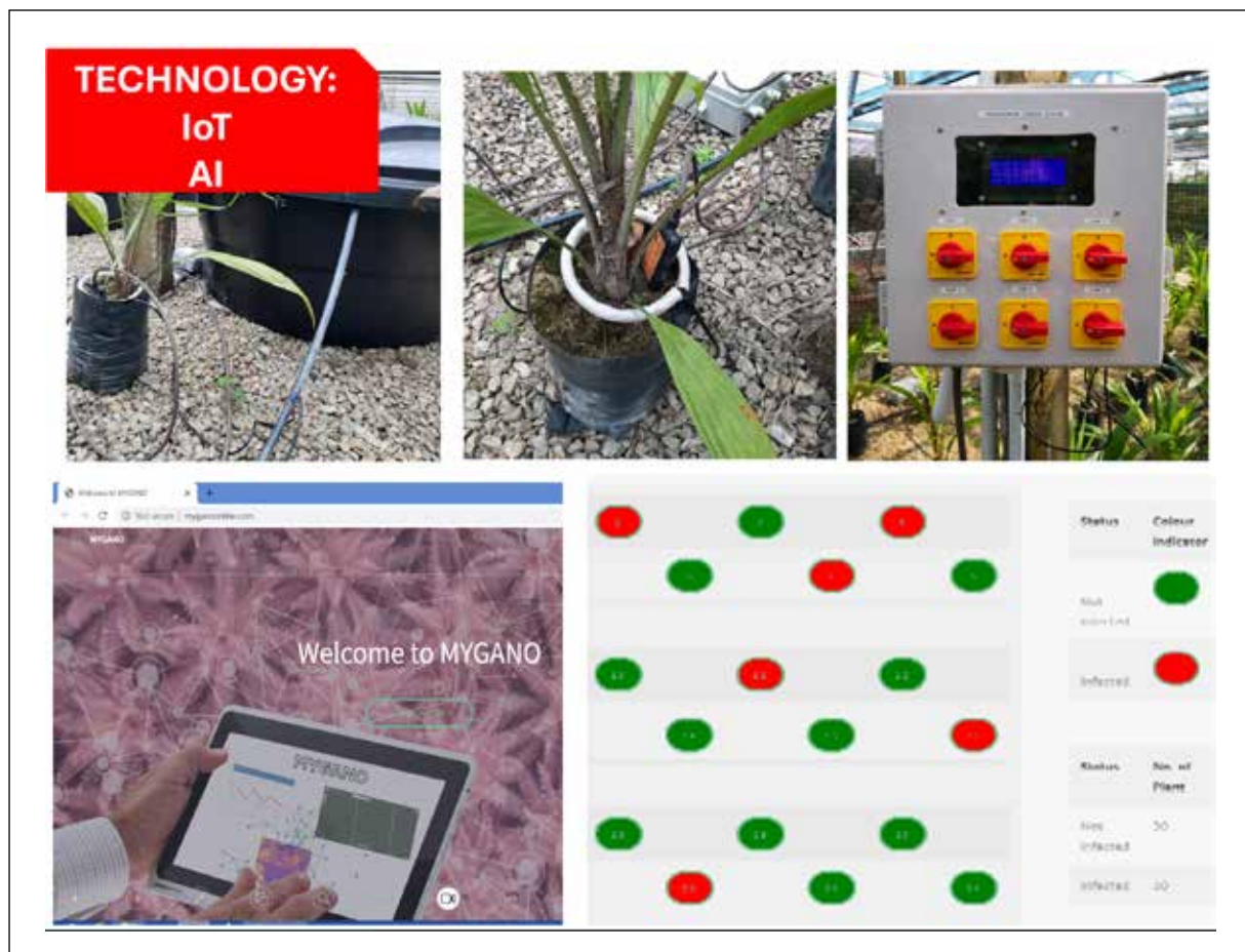
Figure 5: Remote management of oil palm seedlings at nursery using soil sensor, IoT and AI [10].
