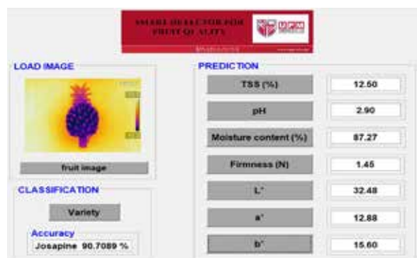
Figure 2: Prediction of quality parameters of pineapple using thermal imaging. Courtesy: Mohd Ali et al. (2022).
